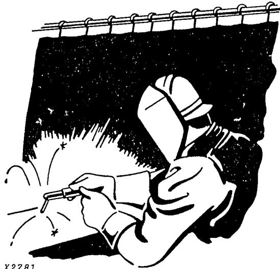
Fig. 174 — Use a Protective Screen To Protect Others From Arc Rays
