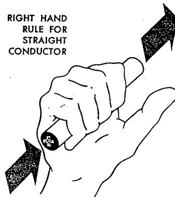
Fig. 22—Right Hand Rule Shows Direction of Lines of Force in a Straight Conductor
