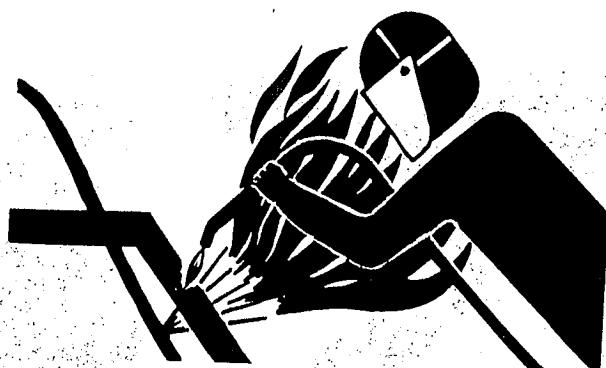
Fig. 106 — Avoid Heating Near Pressurized Lines
