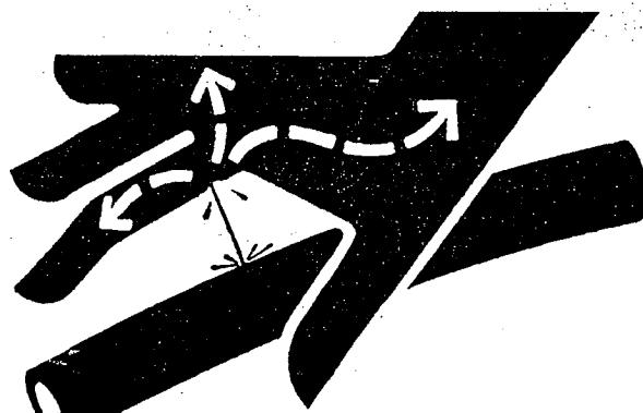
Fig. 104 — Avoid High Pressure Fluids
